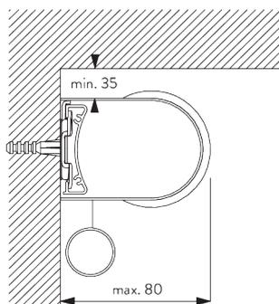
**Installation profile SG 10534 and clamp SG 3044**
