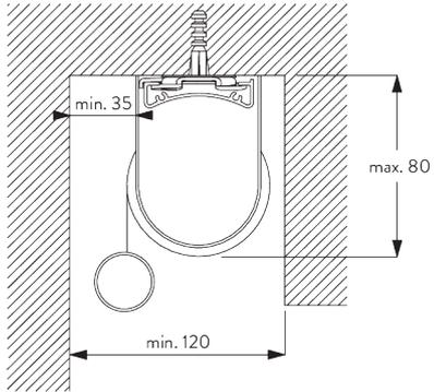
**Installation profile SG 10534 and clamp SG 3044**
