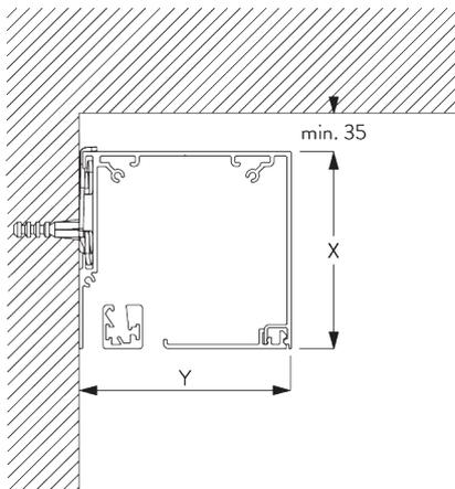
**Box S and clamp SG 3044 / Box L and clamp SG 11180**
