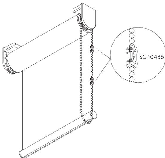
The chain break connector SG 10486 releases the chain should the pulling force exceed 6 kg.
