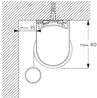
**Installation profile SG 10534 and clamp SG 3044**
