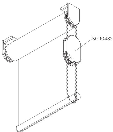
The child safety device SG 10482 releases the chain should the pulling force exceed 6 kg.
